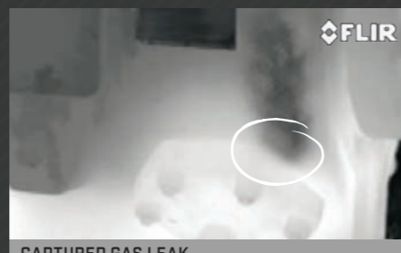
CAPTURED GAS LEAK
