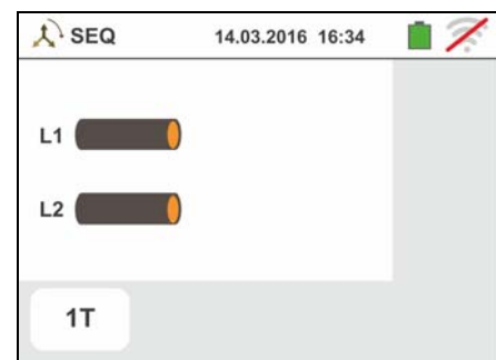
Fig. 24: Phase sequence check of 2T phases with terminal and remote lead
