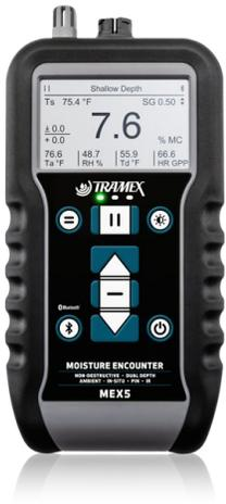
The Tramex Moisture Encounter MEX5 is a digital Dual-Depth, non-destructive moisture meter for wood and various building materials such as drywall, roofing, plaster, tile and masonry. The Moisture Encounter MEX5 has a built-in hygrometer for ambient conditions and psychrometric values, an Infrared Surface Thermometer and also incorporates external in-situ RH probes for in-situ equilibrium RH readings, as well as Pin probes for wood, drywall, and WME readings.
