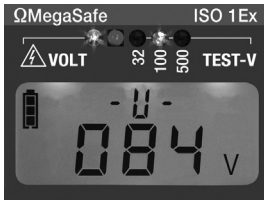
Charge voltage indication with external connected capacitance
