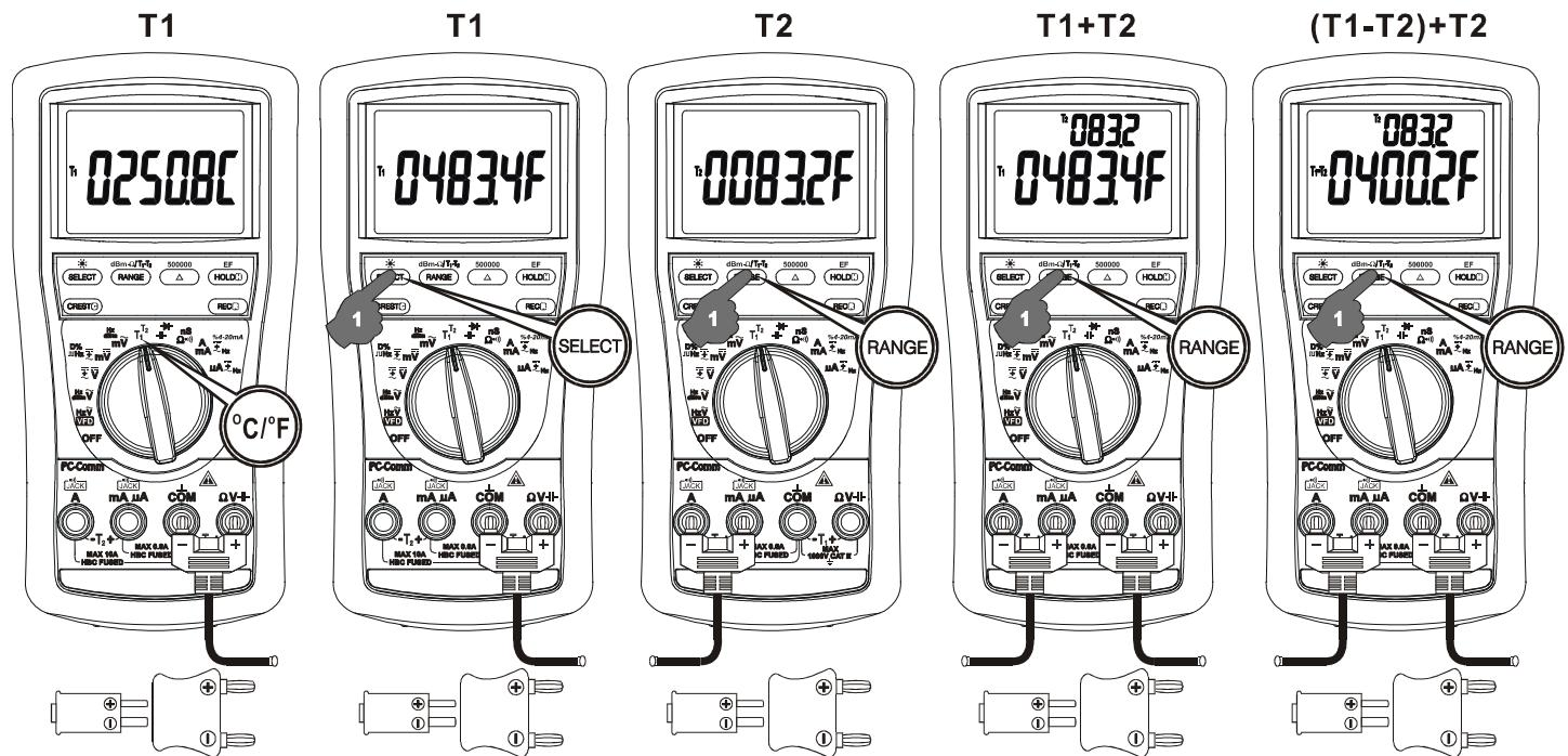
Note: Be sure to insert the banana plug type-K temperature bead probe Bkp60 with correct **+** **-** polarities. You can also use a plug adapter Bkb32 (Optional purchase) with banana pins to type-K socket to adapt other standard type-K mini plug temperature probes.
