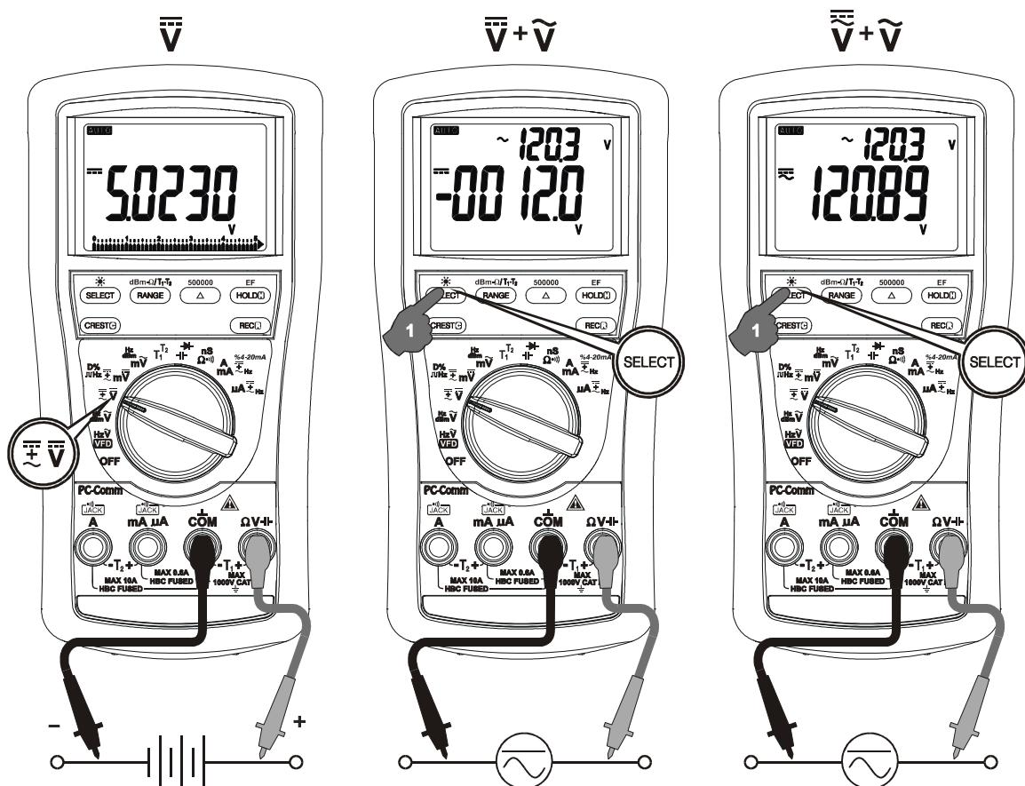
**$DCmV$ ,  $DCmV +ACmV$ ,  $DC+ACmV +ACmV$ , Logic-Level  $\sqcup\sqcap$  Hz, Duty%**
