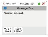
If the instrument detects the absence of the signal to terminal B4 (neutral conductor), it provides the warning screen shown to the side and blocks the execution of the tests
