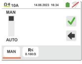
4. Touch the icon to reset the value in the "Ω" field and use the virtual keyboard to set the value of the maximum limit resistance used by the instrument for evaluating the continuity test in the field:  $0.003\Omega \div 0.500\Omega$  in steps of  $0.001\Omega$ . Confirm your choice by returning to the previous screen
