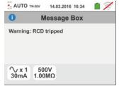
If the instrument detects a danger voltage on PE conductor, it does not carry out the test and displays a screen like the one to the side. This message can also appair in case of an insufficient pressure of the GO/STOP key
