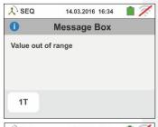
3. If the instrument detects an input voltage frequency exceeding the allowed full scale, it will display a screen like the one to the side.
