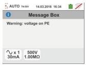
10 If the instrument detects a dangerious contact voltage Ut (over the set limit 25V or 50V) in the starting pre-test, it provides the warning screen shown to the side and blocks the execution of the tests. Check the PE conductor and earth plant efficiency
