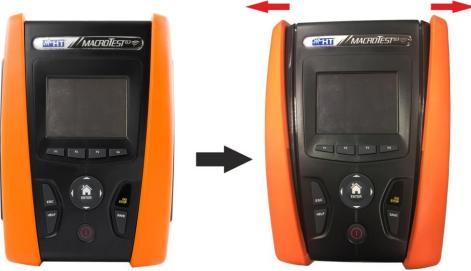
Fig. 40: Remove lateral half-shells
