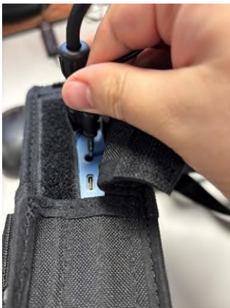
Figure 4.5 Connecting the headphone cable
