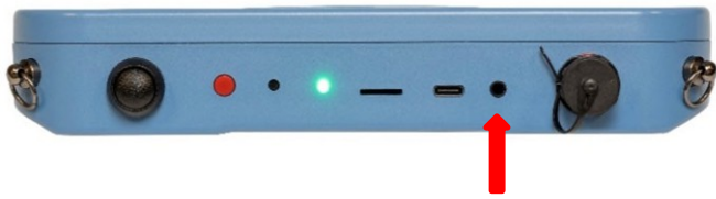
Figure 2.10: Audio socket on the RD510 locator display
