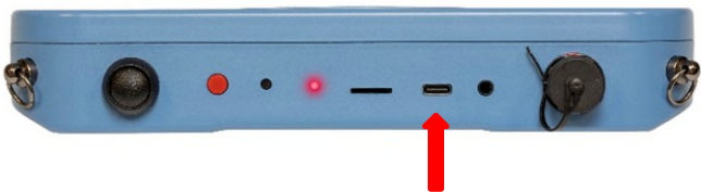
Figure 2.6: Charging socket on the RD510 tracker display
