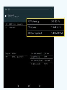
**The rotation speed** of the motor is equal to the synchronous speed minus the slippage. The synchronous speed is equal to the frequency divided by the number of pole pairs.
