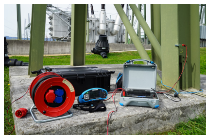
Bundle set with all the accessories in a portable IP67 protected case for field transport.
