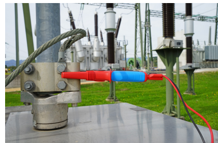
Kelvin Crocodiles ensure robust 4-wire connection for reliable results.
