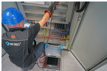
Internal resistance of the Power Source with Automatic trip-out ability evaluation with high accuracy on DC circuits.
