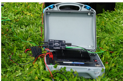
Body resistance simulation with 1 kOhm adapter A1597 for correct Touch Voltage calculation.
