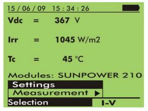
The I-V 400 interface is realized by a menu level structure management which is easy and intuitive
