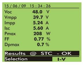
The immediate display of results allows to evaluate the technical features of the modules. **I-V 400** also provides an indication (OK/NO) for the correspondence between the detected and the rated features declared by the manufacturer
