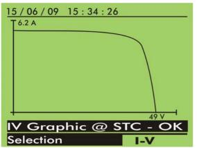
I-V 400 permits to evacuate also by graphical mode the I-V curve of panels both on standard reference (STC) and operating conditions
