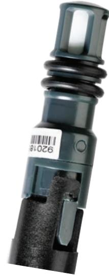
Protimeter Flooring HygroStick BLD4755 is used with Protimeter Flooring Kits to measure and monitor concrete moisture. These probes are installed into a sleeve fixed in concrete and, with the attached cable, measure moisture and Relative Humidity (RH) with Protimeter devices.
