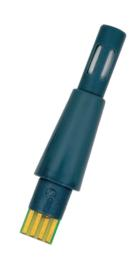
Protimeter HygroStick POL4750 is an analog Relative Humidity (RH) and Temperature Sensor with a unique 8-pin interface for use with Protimeter devices. The HygroStick sensor is ideal for high RH testing with low drift and the ability to recover from dew point conditions. These sensor can be directly attached to the device or through Protimeter Extension Cable BLD5802.
