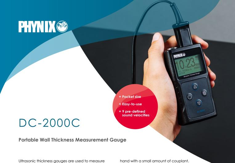
the thickness of materials from one side by means of ultrasound. An ultrasound tranducer generates a high-frequent ultrasound pulse which is sent through the material to be measured. At the backside of the material the pulse is reflected and travels back to the transducer. As the material and its sound velocity is known the travel time of the pulse is used to calculate the material thickness. Wall thickness gauges are often used to determine the amount of corrosion on ships or at pipeline tubes.
