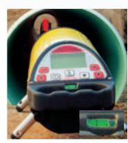
**Automatic grade compensation** with the housing rolled up to  $\pm$  3°, the Piper will compensate and correct for the grade errors.
