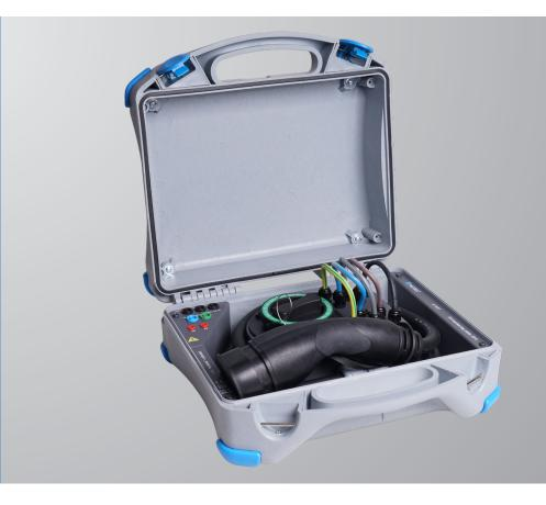
The A 1631 EV monitoring cable is a special accessory designed for CP signal, current and voltage monitoring during Electric Vehicle (EV) charging process in conjunction with supported Metrel testers and adapters. It is equipped with a Type 2 female plug connector to connect to an EV and a Type 2 male socket outlet for connecting to Electrical Vehicle Supply Equipment (EVSE).
