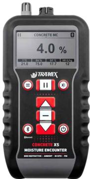
The Tramex Concrete Moisture Encounter X5 is a non-destructive digital multi moisture meter for concrete decks providing instant and precise quantitative measurement of moisture content of concrete using Gravimetric testing as a baseline. The CMEX5 incorporates a built-in hygrometer and plug-in ports for the relative humidity probe and pin-type probe testing of roofing materials.
