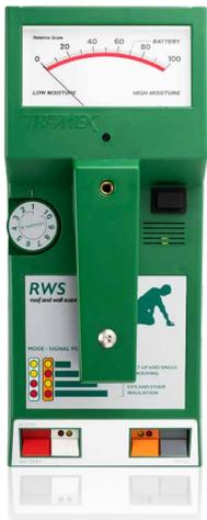
The Tramex RWS Roof and Wall Scanner is a multi-mode non-invasive impedance scanner designed for the instant, precise and non-destructive evaluation of moisture conditions and leak tracing in roofing per ASTM D7954 and in wall systems of the building envelope.
