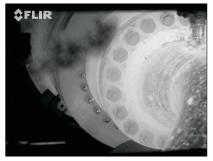
Natural gas leak on compressor valve
