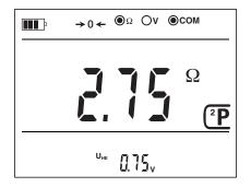
The  $\rightarrow$  0  $\leftarrow$  symbol blinks during the compensation. When it is done, the display unit indicates 00.00 $\Omega$ .
