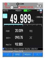
Display of the measurement in % of a logical signal (TTL, CMOS, etc.)
