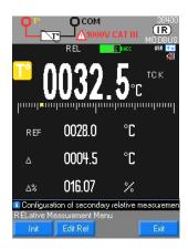
Measurement of the temperature in °Celsius using a thermocouple between the V and COM terminals
