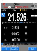
In the "DC" mode, you measure a direct voltage or the DC component of an AC voltage. Selection of the coupling from among:
