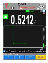
Reading of the threshold voltage; if the circuit is open or the threshold of the diode >4V, the indication is OL.
