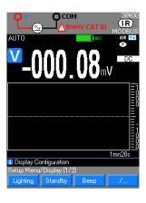
selection of 3 levels of back-lighting of the display unit in order to limit the power consumption of the multimeter, as follows: Eco, Normal, Max
