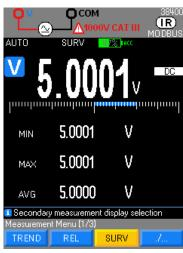
The **SURV** mode (available under **MEAS...**) monitors the variations of a signal, recording the extremes (**MIN** and **MAX**) of the main measurement and calculating its mean (**AVG**).
