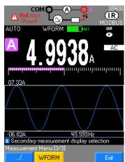
During an AC current measurement, the waveform of a signal at a frequency between 10 Hz and 600 Hz can be viewed using the WFORM function
