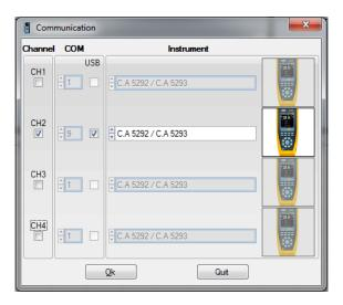
With some Bluetooth adapters, a reboot of the PC is recommended to validate the connection. The connection parameters are specific to each multimeter. They must be assigned manually, the first time only.
