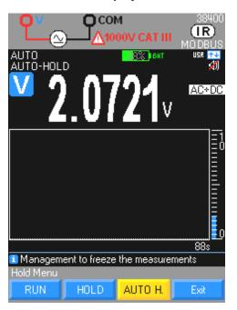
Display of the wiring diagram the terminal block as a function of the measurement Digital display: of the quantity measured, - of the value measured. of the type of measurement, etc. Secondary display: in graphic form or in the form of 3 display units Scrolling information Properties of the F1, F2, F3, and F4 keys
