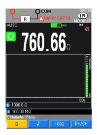
In the 50  $M\Omega$  range, in order to avoid the influence of the mains and guarantee the stated specifications, it is best to disconnect the multimeter from the Wall Plug to avoid perturbations.
