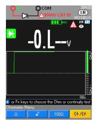
Zener diode or LED: selecting this diode applies the same function as for the diode above but with a maximum voltage of 26V and a maximum current of 10mA.
