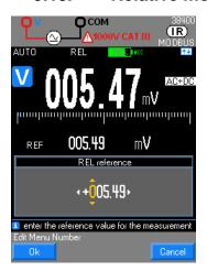
This mode indicates that the value displayed is relative to a reference value. It is available for the following measurement functions: V, Hz, Ohm, clamp, capacitance, temperature, and current.
