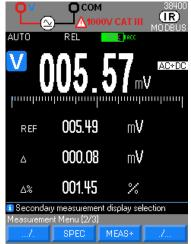
• SPEC : directly displays the tolerance of the measurement in progress; there is no need to search for it and calculate it.
