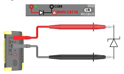
This function performs a diode forward voltage check to verify:
