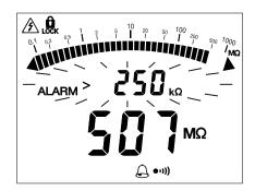
In the example above, the user can thus check that their continuity measurement is indeed less than 2  $\Omega$ , just by listening, without looking at the display unit. They can check insulation quality in the same way.
