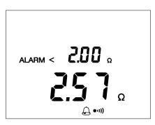
While it is displayed, you can change this value using the  $\blacktriangle$  key, except during insulation measurements. For each position of the switch, there are 3 pre-recorded threshold values:
