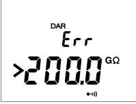
With the C.A 6524 or C.A 6526, if this occurs during a DAR or PI measurement, the instrument interrupts the measurement and displays the screen shown opposite.
