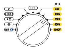
Set the switch to one of the  $M\Omega$  positions.
