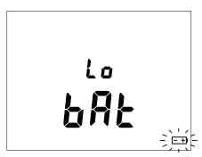
The batteries must then be replaced (see § 4.2), since the battery life indication is no longer reliable.
