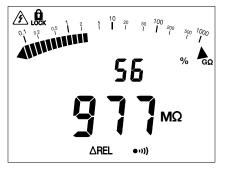
In insulation measurements, only the digital display is modified by the ∆REL. The bargraph continues to display the true measured value.
