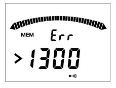
When the memory is full (300 records for the C.A 6524; 1300 for the C.A 6526), it is no longer possible to record measurements and the instrument displays the screen shown opposite.
