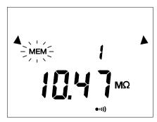
It is recorded with all information tied to it but not necessarily displayed at the time of storage: voltage, current, duration of tests T1 and T2 in the case of PI and DAR, etc.
