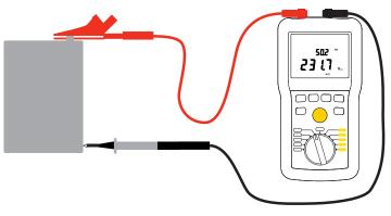
The instrument displays the voltage on the terminals. It detects whether the voltage is AC or DC and, if it is AC, displays its frequency (on the C.A 6524 and the C.A 6526).
