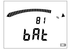
If the battery voltage is too low to ensure correct operation of the instrument, it so reports.
