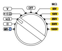
As for a continuity measurement, connect the device to be tested to the terminals of the instrument. The device to be tested must not be live (see 2.4.3).
