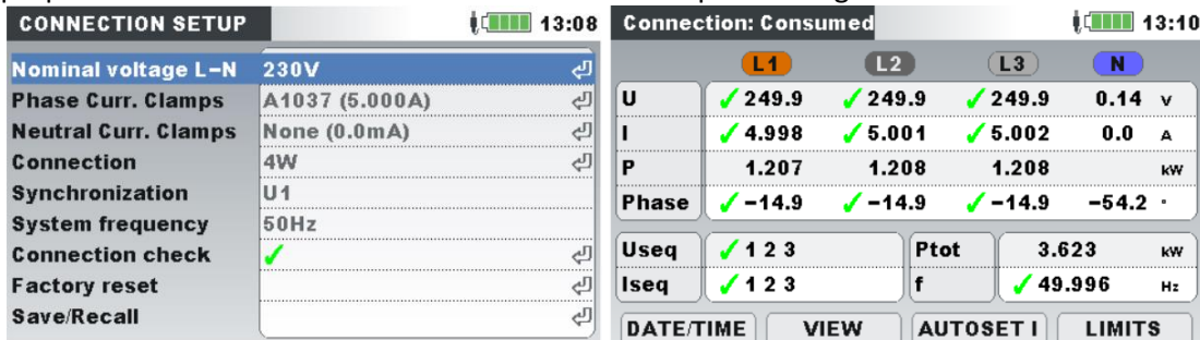
Figure 76: PQA setup connection and Connection check
