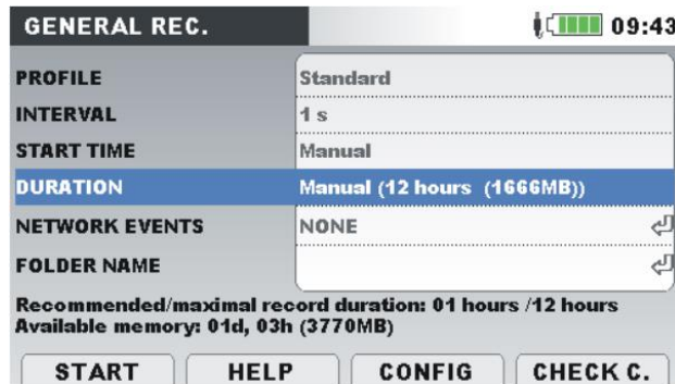
Figure 180: General Recorder setup to allow auto-recording restart, when reaches maximum file length
