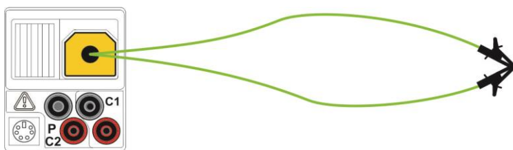
Figure 5.10: Shorted test leads
