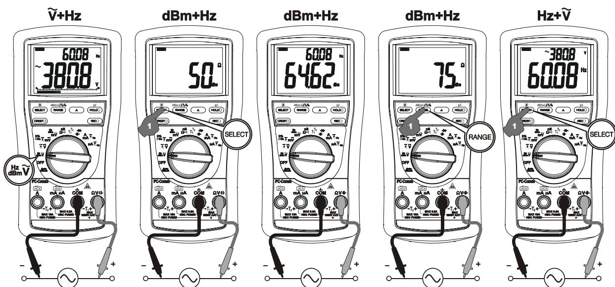
**Note:** Hz Input sensitivity varies automatically with voltage (current function alike) range selected. 1V range has the highest and the 1000V range has the lowest. Auto-ranging measurements normally set the most appropriate trigger level. You can also press the **RANGE** button momentarily to select another trigger level (voltage range) manually. If the Hz reading becomes unstable, select higher voltage range to avoid electrical noise. If the reading shows zero, select lower voltage range.
