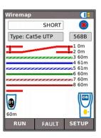
Fig 21 Short circuit by pin
