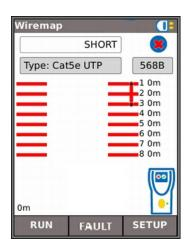
Fig 19 Short circuit by pin
