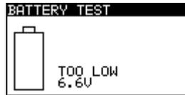
Figure 1.1: Discharged battery indication
