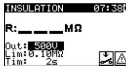
Figure 6.21: Insulation resistance starting screen
