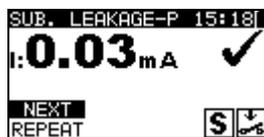
Figure 6.28: Substitute leakage - P result screen
