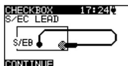
Figure 4.14: S/EB test lead check starting screen
