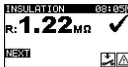
Figure 6.22: Insulation result screen
