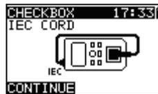
Figure 4.15: IEC test cord check starting screen
