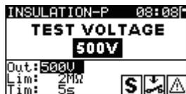
Figure 6.9: VDE Organizer autotest – Insulation resistance - P starting screen
