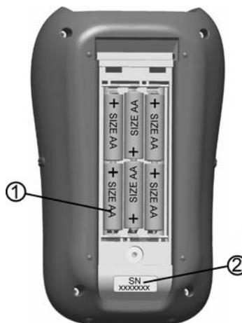
Figure 2.4: Battery compartment
