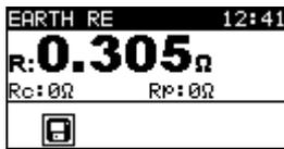
Figure 6.1: Typical display in earth resistance function
