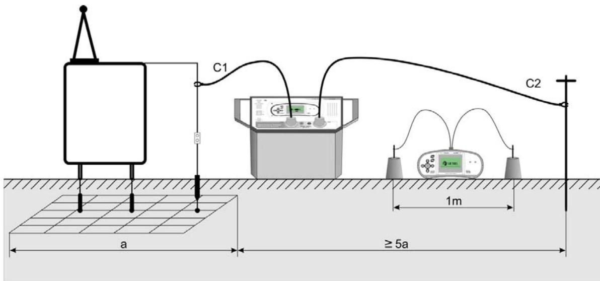
Figure 7.2: Step voltage measurement
