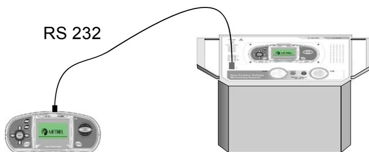
Figure 7.8: Connection of the instruments during synchronization
