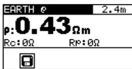
Figure 6.2: Typical display in specific earth resistance function
