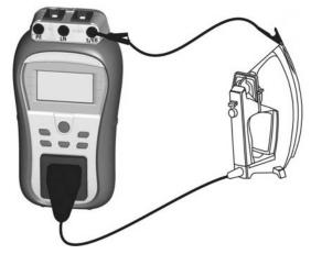
Figure 5.5: Measurement of Earth continuity
