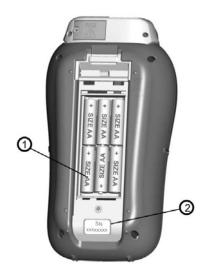
Figure 2.4: Battery compartment
