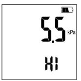
Auto:automatic selection of the measurementLo (Low):low measurement range (high resolution)HI (High):high measurement range (low resolution)
