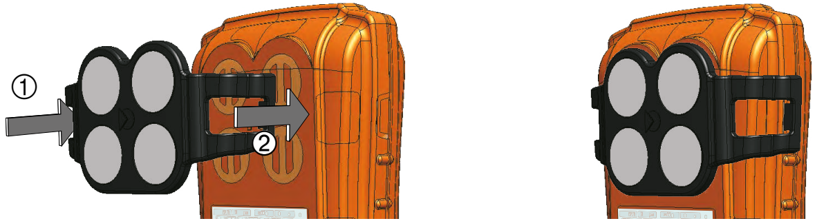
Figure 6: Fitting the external filter plate
