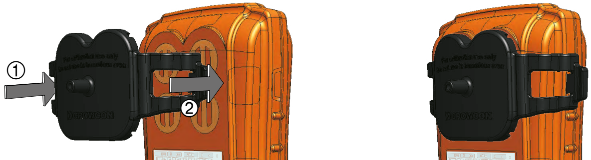
Figure 5: Fitting the calibration/bump test plate
