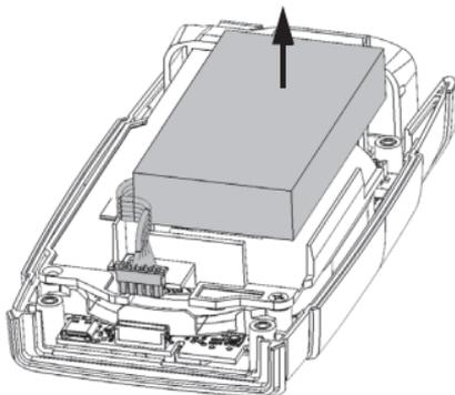
7. Place the new battery so that its wires are located on the left side, toward the front.
