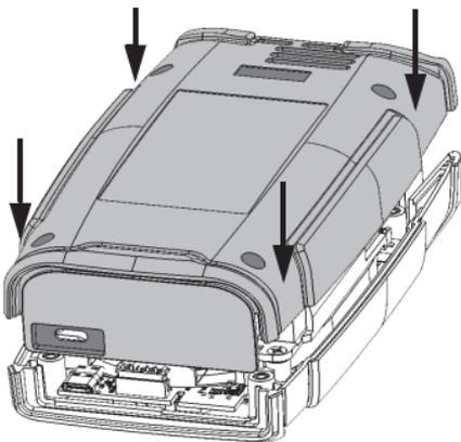
11. Using a 2.5 mm hex socket screwdriver, turn the screws (4) clockwise until they are tightened.
