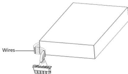
8. Push the new battery toward the bottom of the case until it stops.
