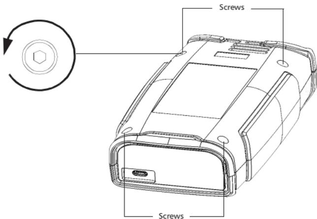
4. Hold the back panel by its sides and pull it up to remove it.
