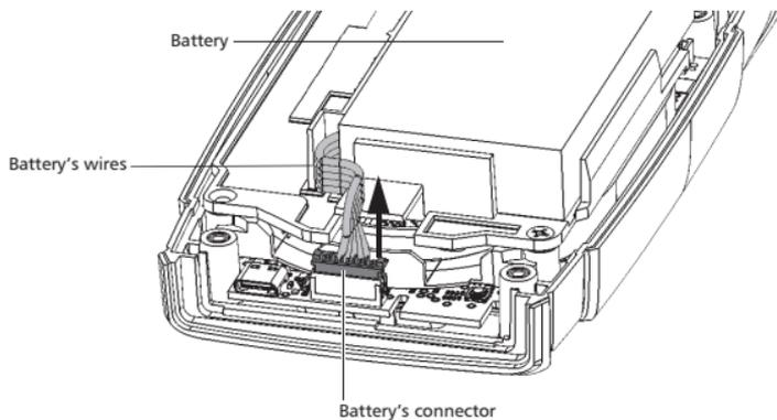
6. Pull the battery up to remove it.
