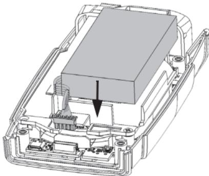
9. Ensure that the battery's wires are *above* the plastic tab (not under), and then connect the battery's connector to the corresponding socket.
