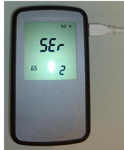
Figure 3-2: To the left: a picture of the SW screen after it has auto-detected a monitor plugged in the USB port. To the right: the monitor shows a LCD-screen similar to this picture when it is plugged into the PC. The serial number of the monitor in the form SEr-65-2 is shown. (The numbers will be different on different monitors).
