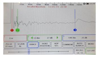
At this time, you can change the parameters of the presented waveform such as the pulse width, vertical gain, range and VOP. You can move all the 3 cursors and measure distances to multiple events on the cable.
