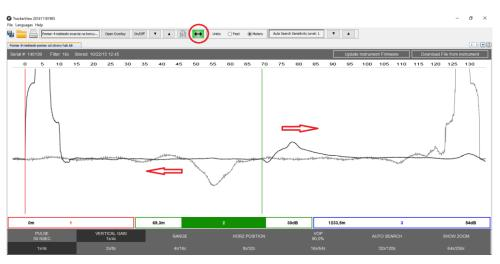
Note: Both features: ""Mirror Horizontal"" and ""Drag Overlay Waveform" are active only when you overlay waveforms (compare two graphs on the screen).
