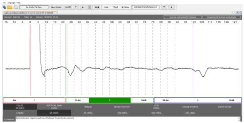
While testing a cable - when the end of the cable is disconnected from the cable plant, the largest reflection will be the end of the cable and therefore cursor No. 3 will move to the end. If not disconnected, the blue cursor will move to the largest impedance mismatch on the cable line.
