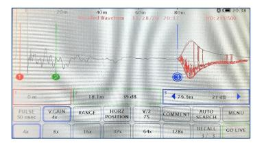
NOTE: Due to its nature, IFD testing can take some time. In order not to lose the measurement data due to the internal battery run time level, please, make sure you control the charging status of the battery. You can always activate IFD mode with the charging procedure on (the active use of the TDR during the charging procedure from the 230 V AC mains or from the external power generator).
