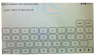
NOTE: Any comment that has been entered by the user will be visible for the procedure of transferring the data to a PC (data transfer screen). The comment will be transferred with the file and the user can find it in the Comment area on the TrackerView screen while viewing the waveform on a PC.
