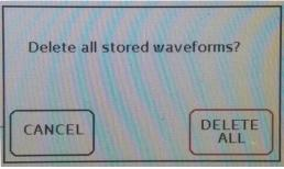
4. If you have pressed DELETE ALL, the next step is to confirm your wish to continue the procedure of deleting all the measurement data by pressing YES or you pressing NO (to stop the deleting procedure).
