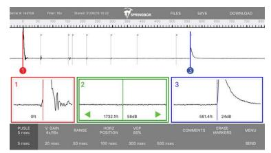
You can find **"Auto-Search Sensitivity Level"** control option in the MENU at Settings. You can adjust the level of sensitivity used for the "Auto-Search" mode, where Level 1 means "automatic search for less severe faults" and Level 5 means "automatic search for more severe faults".
