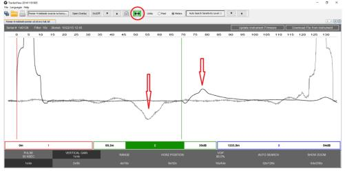
In order to complete the procedure of correct interpretation of such fault analysis, the user needs to use one more feature – "Drag Overlay Waveform". You just click on the "Drag Overlay Waveform" icon on the Upper Tool Bar and then use the mouse to drag the overlay waveform left or right until you get the expected results.
