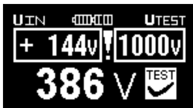
Fig. 3.10a Example of USPD measurement result (discharging in progress)
