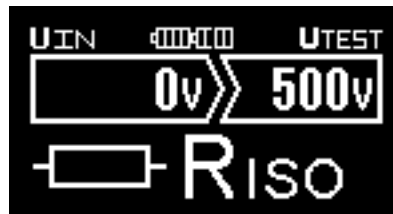
Fig. 3.5 Example of setting for insulation resistance measurement
