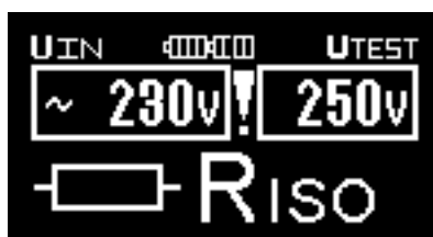
Fig. 3.1 Example of voltage measurement
