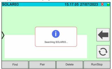
Fig. 16: Pairing a SOLAR03 remote unit - Step 2
