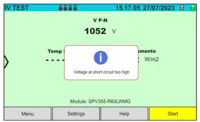
If, during the execution of an I-V or IVCK measurement, the value of the measured voltage is greater than 12%Voc, the instrument does not carry out the measurement and displays the message shown in the screen alongside. Check the circuit being measured and repeat the test
