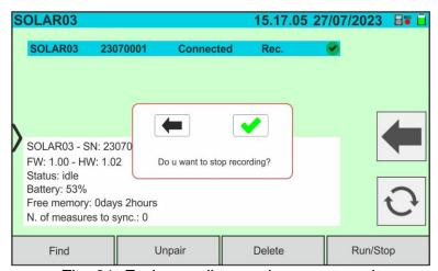
Fig. 21: End recording on the remote unit
