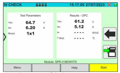
Fig. 60: IVCK test result @OPC with synchronous recording
