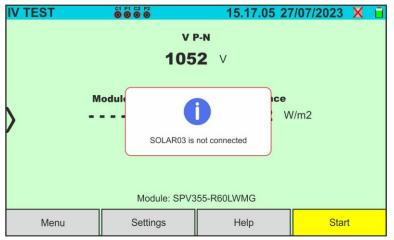
If the SOLAR03 remote unit is active but **not connected and not recording**, the instrument does not perform the test and displays the message shown in the screen alongside. Connect the SOLAR03 remote unit
