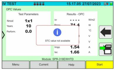
If, during the execution of an I-V or IVCK measurement, the instrument is unable to determine the @STC values, it displays the message shown in the screen alongside. Check that you have stable irradiation, in addition to the correct exceeding of the minimum threshold and that you have carried out the measurement in accordance with the indications of the M304 accessory
