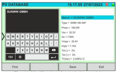
Fig. 28: Modification of an existing module
