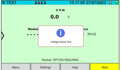
If the instrument detects a voltage of -0.5V≤VPN≤15VDC at the P-N terminals of the string, it does not perform the test, emits a prolonged audible signal and displays the message shown in the screen alongside. Check the tension on the string
