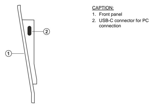
Fig. 2: Description of the instrument's side
