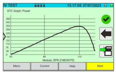
Fig. 40: Example of power measurement result - STC curve
