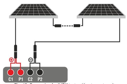
Fig. 45: Connection for IVCK tests without remote unit
