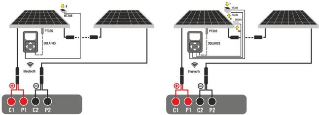
Fig. 52: Connection with remote unit SOLAR03 on Monofacial and Bifacial modules
