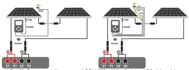
Fig. 33: Connection with remote unit SOLAR03 on Monofacial and Bifacial modules
