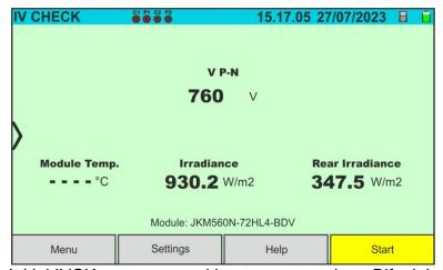
Fig. 54: Initial IVCK test screen without remote unit on Bifacial modules
