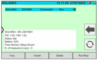
Fig. 42: Recording Activation on Remote Unit - Step 2
