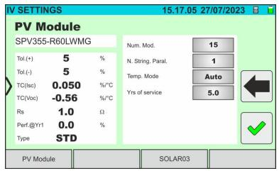
Fig. 36: I-V curve measurement parameter settings
