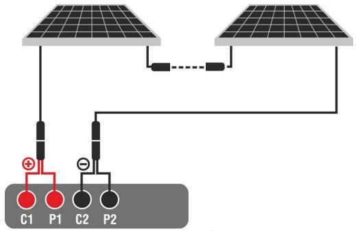
Fig. 13: Instrument connection for DMM Function
