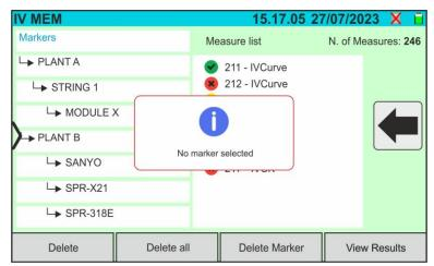
If an attempt is made to delete a marker with the word "Markers" highlighted, the instrument will display the message shown in the figure and will not perform the operation. Select a valid marker
