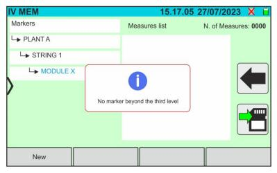
When the third-level marker is selected, touching the "New" key will display the screens shown in the figure and the instrument will not perform the operation. It is not possible to define markers beyond the third level
