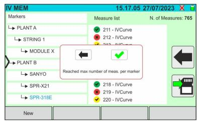
If, during saving, you try to associate a measurement with a marker in which the maximum number of possible measurements are present (max 500), the instrument shows the message shown in the figure on the side and does not carry out the operation. Download the measurements to the PC and delete them before saving again
