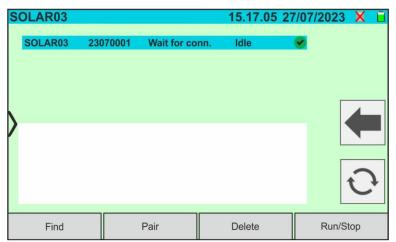
Fig. 17: Pairing a SOLAR03 remote unit - Step 3
