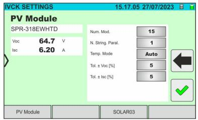
Fig. 55: I-V curve measurement parameter settings
