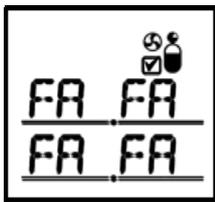
If the calibration fails, the phrase FA(Fail), not OK, appears on the LCD. Press the button to enter the initial fresh air calibration mode and if you do not press the button, it changes into the measuring mode. If FA continues, please consult SENKO or the store you purchased as it may require the replacement of the sensor or repair of the device.
