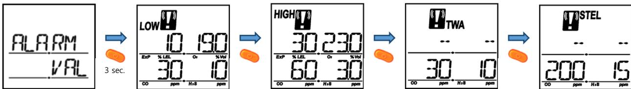
Press the KEY button (
