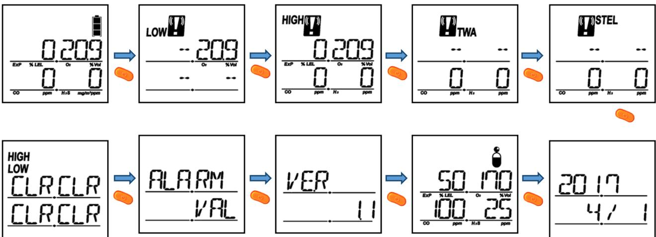
The displays in ten different modes as above are shown in the measuring mode every time when you press the KEY button(
