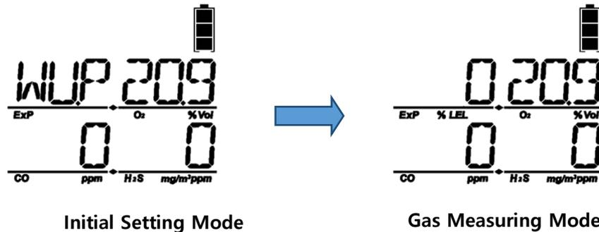
Once activated, the device will enter the warm up stage to stabilize sensors. The warm up process is completed, the device is ready to detect gases.
