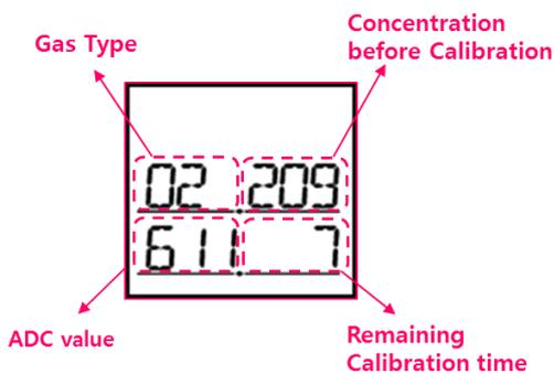
**Initial Standard gases concentration for calibration**
