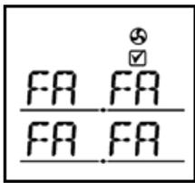
If the calibration fails, FA(Fail), not OK, appears on the LCD. Press the button to enter the initial fresh air calibration mode and it changes into the measure mode if you do not press the button for 3 seconds. If FA continues, please consult SENKO or the store you purchased as it may require the replacement of the sensor or repair of the device.
